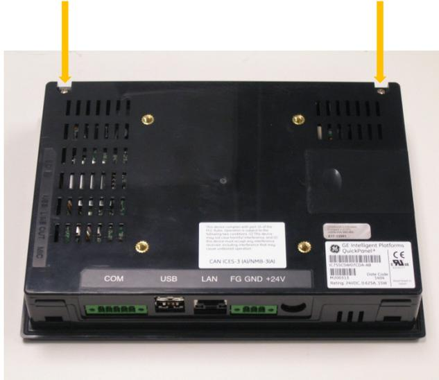
2. Remove the battery cover from the back of the unit and remove the battery
