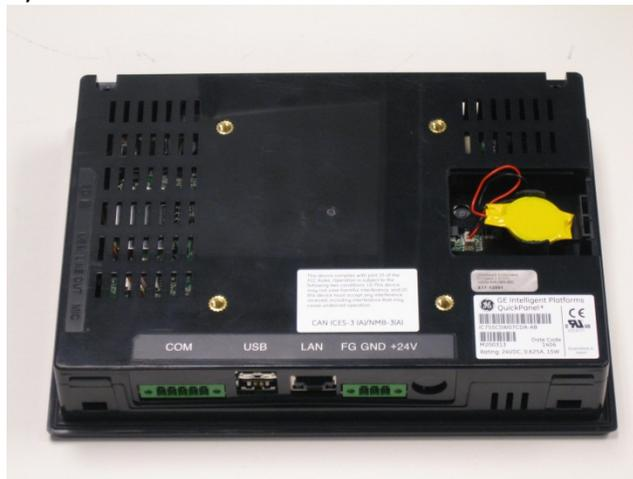
3. Carefully remove the back cover by lifting on the end where the screws were removed. At the same time, gently pushing downwards to clear the I/O connectors.
