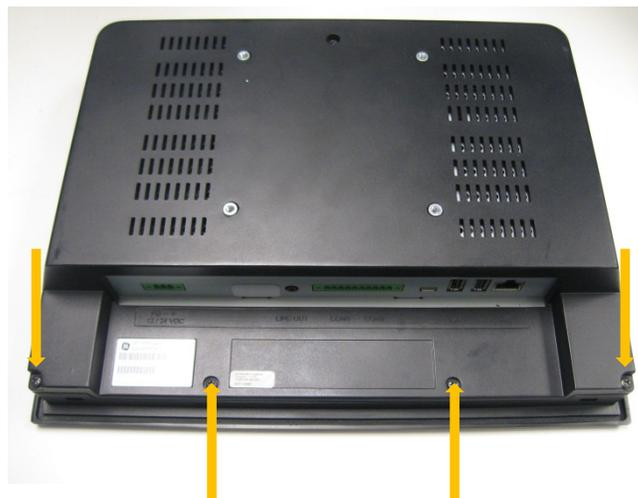
2. Carefully remove the plastic back cover. (On 10", 12", and 15" QuickPanel+, plastic side tabs may need to be gently depressed to release the catch mechanism).
