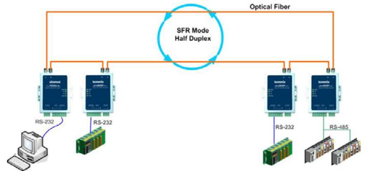
When the JetCon 2401 is working at SFR mode, there are some signal latencies will be caused by the device and the fiber cable. The following information will indicate those parameters for the link node and distance calculation.
